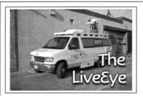
CKCO's "LiveEye" microwave truck enables us to broadcast live from the scene of the action almost anywhere in the local area, and as far away as London. Video and audio signals are transmitted by microwaves from the mast on the top of the van. This mast can rise 60 feet (approximately 20 metres) straight up from the top of the van. The signal is received by an antenna on the top of a nearby apartment building, and brought into the station, from there, by a fibre-optic cable.
